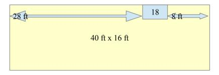
Baseboards 18 and 6 have 2 sets of trestles, so start with 18 at the back. (It's not practical to start from board 6.) Left side 28 ft from left end, right side 8 ft from right end. Then 19 to 24 and 17 to 7 at the same time. Finally 6 on 2 trestles, followed by 5 to 1 connecting to 24.
